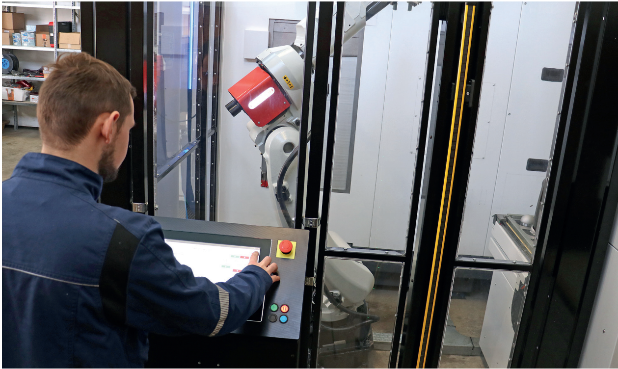
The robot-assisted tower solution from RoboJob teamed with the Emco Maxxmill 750 makes it possible to machine parts around the clock.
